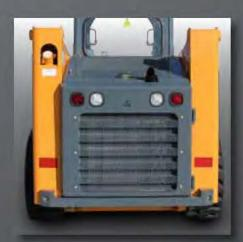
optional and boost the rated load capacity to 2,110 lbs. (957 kg) on the 1900R, 2,370 lbs. (1075 kg) on the 2200R, and an impressive 2,780 lbs. (1261 kg) on the 2600R.
