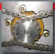
HEAVY-DUTY DRIVETRAIN is composed of durable components, including zero-maintenance axles. Adjustments can be made to the chain system from outside the unit.
