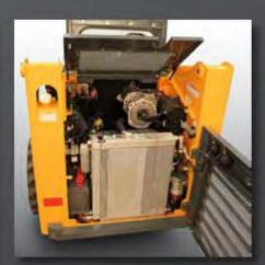
QUICK SERVICE is made possible with a swing-open rear door, flip-up engine cover, and tiltable ROPS/FOPS that fully exposes maintenance points at the engine, battery, and filler caps.
