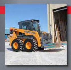
SPEED UP ... with maintenancefree, radial-piston drive motors with high start-up torque and maximum ground speeds up to 12.5 mph<sup>1</sup> (20 km/hr) for quick acceleration.
