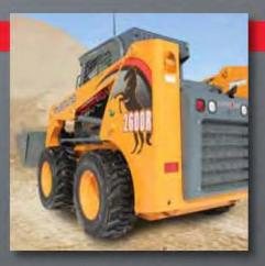
SMOOTH RIDE ■ is achieved with a longer wheelbase and low center-of-gravity. The HydraGlide<sup>TM</sup> ride control option provides stable operation over uneven surfaces.
